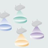
Access Ports with Virtual AP (One Access Port Supports Four Virtual LANs)
