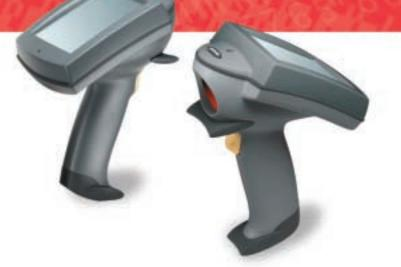
upward and backlit for comfortable viewing. The display and its convenient built-in touch screen with virtual keyboard are encased in tough polymer that protects them from dust and moisture. The terminal grip has a futuristic handle-forward design and ergonomic contours that fit the hand snugly. At the first stage, the trigger activates the screen, at the second, the scanner.
