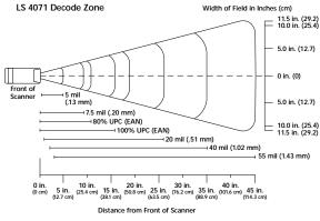
Decode zone measurements are based on an integrated LS 400X scann-high quality bar codes at 73°F/23°C. Discrete LS 4000 scanner performa vary slightly depending on interface controller or portable terminal be
