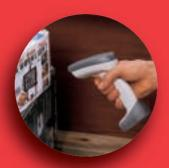
The LS 4071 cordless scanner is ideal for scanning items too heavy or bulky to place on the checkstand.
