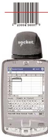
The CF Scan Card 5P brings a new level of portability and performance to mobile data collection by combining Socket Mobility Friendly™ CompactFlash technology with a powerful Class 2 laser scanner engine from Symbol Technologies that is also the smallest and lightest laser scanner engine in the world.
