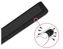
Note: Your device's internal antenna is located along the bottom back of the device. Do not block the antenna; doing so may affect signal quality and may cause the device to operate at a higher power level than is necessary.
