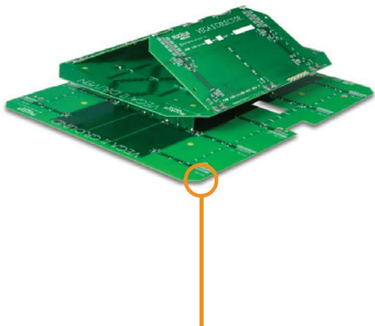
A patented, sectorized smart antenna array in each ZoneFlex 7762-S outdoor AP integrates horizontally and vertically polarized high-gain, directional antenna elements to provide 24 potential signal paths to any given end device while delivering up to 10dBi in signal gain and up to 15dB of interference avoidance within a 120 degree azimuth for unprecedented range extension, signal reliability and higher data rates.
