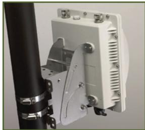
Pole-mounting can be performed in minutes with all configuration and management performed centrally
