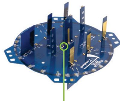
A patented smart antenna array integrates six high-gain vertically and horizontally-polarized antenna elements. This enables up to 4096 potential antenna combinations and up to 10 dB gain, delivering unprecedented range extension, signal reliability and higher data rates.
