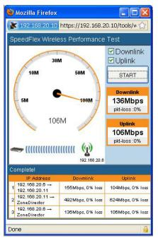
SpeedFlex<sup>™</sup> is a unique wireless performance test tool integrated within the ZoneFlex<sup>™</sup> family of centralized controllers that measures the Wi-Fi throughput of associated wireless LAN clients.
