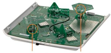
BeamFlex+ Adaptive Antenna Technology
