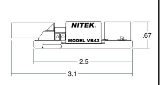
Video Balun-Combiners<sup>™</sup> for twisted pair up to 1,000 feet (750 feet when used with DVR equipment) in conventional UTP applications, 100 meters in TIA/EIA 568 applications.
