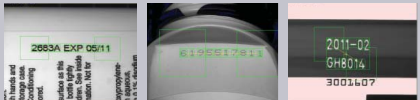
Date/Lot code examples: hot stamped, ink jet, laser marked, plus multiple inspection performed in one system
