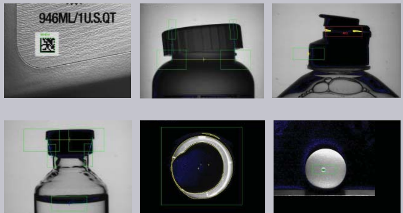
Inspection examples: label presence and skew, label correctness, cap skew, open cap, fill level and crimp inspection, safety seal inspection, tablet hole presence
