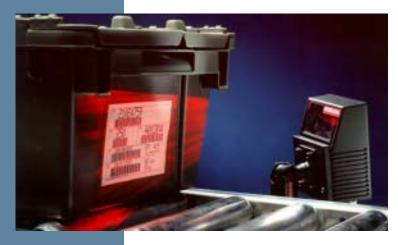
the operating life and temperature, laser current levels, and frequency of power-ups—help prevent costly downtime. For example, user defined messages alert the operator when thresholds have been exceeded and allow for intervention before problems arise.
