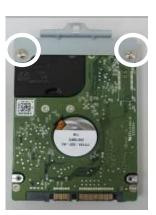
Remove the HDD screws (x3).
