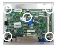
4. Remove the screws (x5) on the Motherboard.
