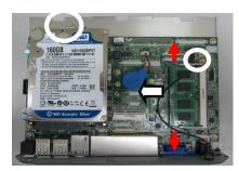
3. Remove the HDD screw (x1) and remove the memory and LED cable.
