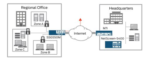
The SSG550M deployed at a branch office for secure Internet connectivity and site-to-site VPN to corporate headquarters. Internal branch office resources are protected with unique security policies applied to each security zone.
