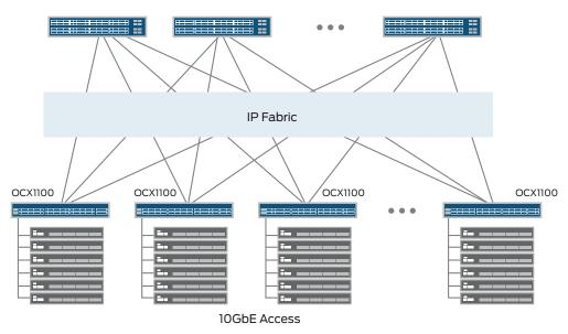
Figure 1: IP fabric deployment using the OCX1100
