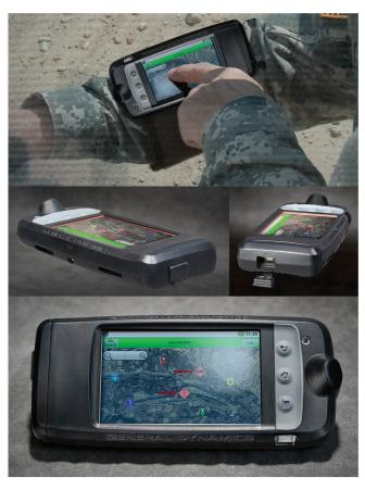
The General Dynamics Itronix rugged, wearable GD300 computer provides state-of-the-art ARM® Cortex™-A8 processing power to optimize battery life and performance in an ultra-thin, lightweight casing for real-time situational awareness. With dismounted usage in mind, it is designed to operate for more than 8 hours providing the user access to real-time information anytime, anywhere.
