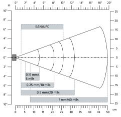
\* The reading distances given are typical reading distances measured in an office environment (200 lux)
