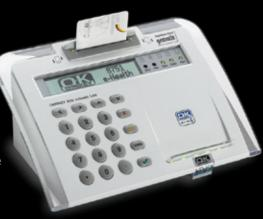
Developed to fulfill the demanding requirements of the German eHealth infrastructure, the OMNIKEY<sup>®</sup> LAN Smart Card Terminal combines the advantages of contact and contactless smart card security with the flexibility and connectivity of Local Area Networks (LAN).
