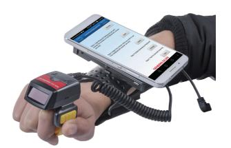
GS WT1000 smart wearable data terminal is specially designed for picking and sorting application. It integrates with wearable armband, ring barcode scanner, smartphone battery charger, data communication function into one device. Your workers will experience the advanced mobile computing and scanning technology with Generalscan smart wearable Android data terminal.
