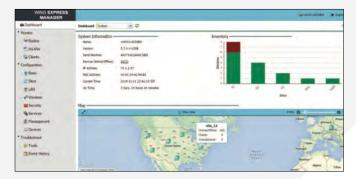
The system-level dashboard presents a map view of all the sites with inventory details for immediate visualization of the entire network. The site-level dashboard allows you to see the status of your access points and their radios, the client devices — including device type — connected to your access points, how much capacity is available, and more. And a drop-down box allows you to view information for your preferred timeframe — the last 30 minutes, the past two hours, or the last 24 hours.
