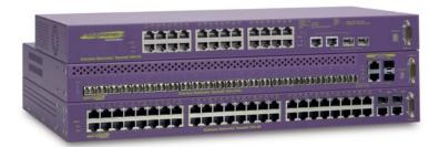
Summit 200 series 24- or 48-port 10/100 and the 24 port 100FX Ethernet switches deliver high-performance, advanced intelligence and features in a compact, low cost package.
