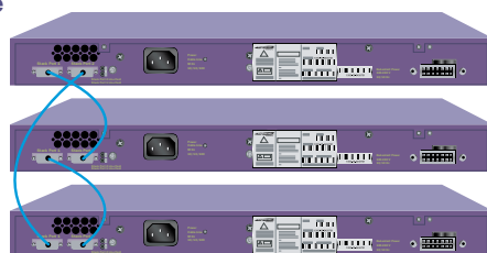
Figure 1: Summit 400-24p UniStack Stack Cabling Illustration
