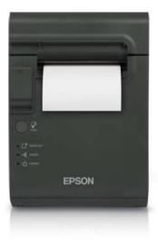
The TM-L90 Plus liner-free compatible label printer delivers all the features you need to print "stay stuck" labels quickly and easily. It prints labels at a speed of up to 90mm/second and receipts at up to 170mm/second at a crisp 203 x 203 dpi, supports variable length label output and accepts label rolls up to 4" in diameter. It is approved for use with the Epson Tested Media.
