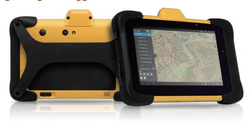
The DT307GS GNSS Tablet features the integration of a brilliant 7" capacitive touch screen and a quad-core, energy efficient processor within a slim, lightweight and durable package. With its high-accuracy GNSS module, Android operating system and optional camera module, this tablet is compatible with existing GIS software for surveying and mapping applications and brings together the advanced workflow for GIS data capture, accurate positioning, and data transmitting.
