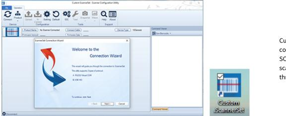
Custom **ScannerSet**: configuration software for SCANMATIC range scanners (programmable through cable)
