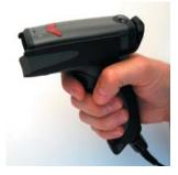
Wireless readers are available with a Bluetooth<sup>®</sup> Class I radio (with a range of 300 feet /100 meters) or Class III radio (30 feet / 9.5 meters) with Bluetooth firmware V1.2; the firmware is easily upgradeable in the field. The CodeXML Bluetooth Modem enables simplified wireless transmission of captured data to a host computer or system. Code's JavaScript Software Development Kit provides programming tools for integrating captured data into enterprise software.
