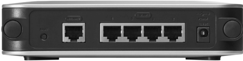
Figure 2. Cisco RVS4000 Gigabit Security Router Port Connections
