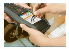
The 8,89 cm transflective colour LCD is produced by CASIO. A user friendly data input and signature capturing method can be done with the touch pen and scratch-resistant touch screen of the device. No matter if glaring sunlight or night delivery – the graphic display with 240x320 pixels is readable under all light conditions.
