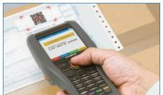
WWAN (EDGE, GPRS, GSM), WLAN (IEEE802.11b/g) and Bluetooth. In addition the actual position can be displayed via GPS. This is the ideal basis for the improvement of service quality, increase of efficiency and reduction of petrol costs.
