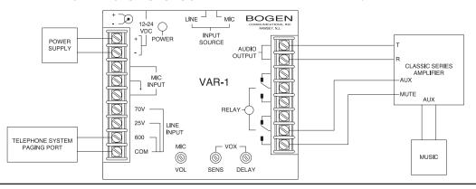
VAR1 used in a security system to activate an amplifier, CCTV, and light relay control.
