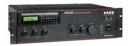
**Description** The Bogen DRZ35 is a unique, self-contained 4-zone music and paging system for small- to medium-sized applications. It combines a digital AM/FM tuner with MIC, LINE, and AUX inputs. It has a 35-watt amplifier capable of driving 4-ohm speaker systems as well as 25- or 70-volt distributed systems.
