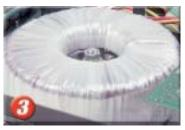
The Black Max power transformer weighs in at 17 lbs. with 2k VA of power (enough to drive most power tools). Size matters in this case, because using a transformer this large keeps core temperatures low, resulting in high reliability and long life.
