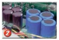
**74,600 µf of capacitance** filters the 110V DC power supply rails creating enormous energy reserve for low distortion, full power bass. The capacitor's 105° F temperature rating ensures long life even under the most harsh conditions.
