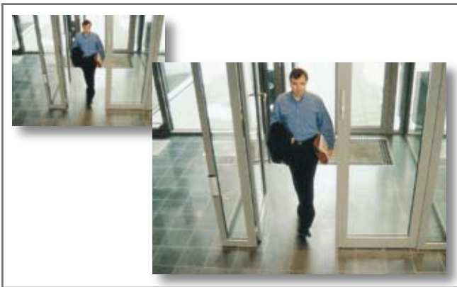
Interlaced scan, 20 ms difference between odd and even lines
