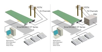
The **SmartWORKS™ DT** provides trunk termination and call control on digital T1/E1 networks. Call Progress Monitoring (CPM), DTMF detection, voice play/record, and barge-in features makes this blade an invaluable resource for interactive telephony applications.
