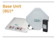
The Base Unit is installed at one end of the PTP link and connects to a central server or to the Internet. The BU is composed of two parts - a universal indoor unit (IDU) and an outdoor unit (ODU). By combining the radio and the modern in the outdoor unit, BreezeNET B offers a true outdoor device with no power loss associated with expensive indoor/outdoor RF cables.
