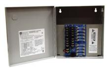
• DC Wall Mount CCTV Power Supplies provide 6VDC to 15VDC distributed via eight (8) Class 2 Rated fuse or PTC protected power limited outputs for powering CCTV Cameras, heaters and other video accessories.
